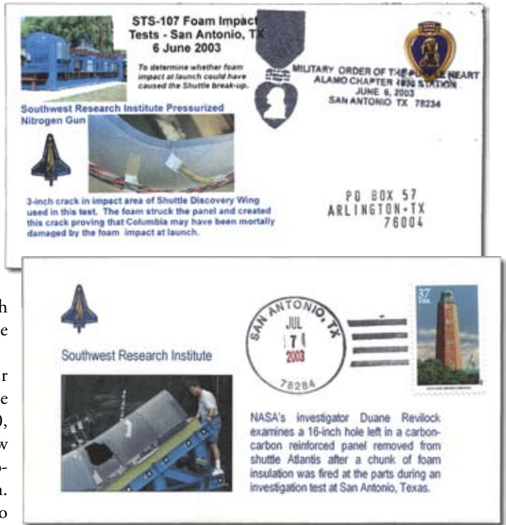
Tests conducted at the Southwest Research Institute in San Antonio, Texas, determined that a piece of foam insulation hit the left wing of Columbia during launch, sealing the shuttle's fate.
