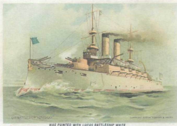
Figure 6: A postcard illustrating KENTUCKY at the time she sailed with the Great White Fleet on their around-the-world voyage 1907 - 1909. Note the 8-inch gun turret bolted directly onto the top of the 13-inch main gun turret.
